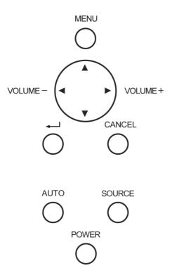
To open the OSD, press the Menu button on the OSD control panel or remote control. There are six initial menus. Press the cursor ▲ or ▼ buttons to move through the initial menus and ◄ to enter the desired menu.
